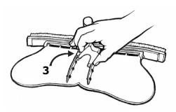
3 - Tilt and lift - the bracket will easily pop out of position. To replace the bracket, position one pin in the hole and repeat the process, pushing down to get the opposite pin into place.
